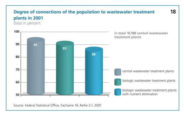
Characteristic of the high standard is also the number and the equipment of the 10,188 wastewater treatment plants. The following bar chart shows the situation in Germany.
